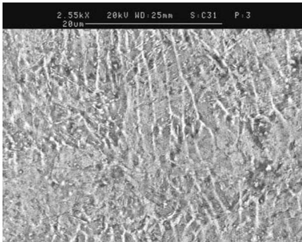
Figure 4 Microstructure of single-pass laser weld metal region of the 1.2343 steel grade.
