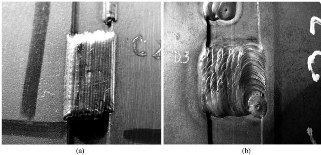
Figure 1 Macroscopic views of the welds: (a) multipass Nd-YAG deposit, (b) multipass GTAW deposit. Groove width corresponds in both cases to 10 mm.
