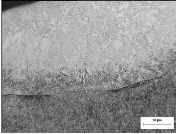
Figure 3 Microstructure of single-pass laser weld metal region of the 1.2311 steel grade.
