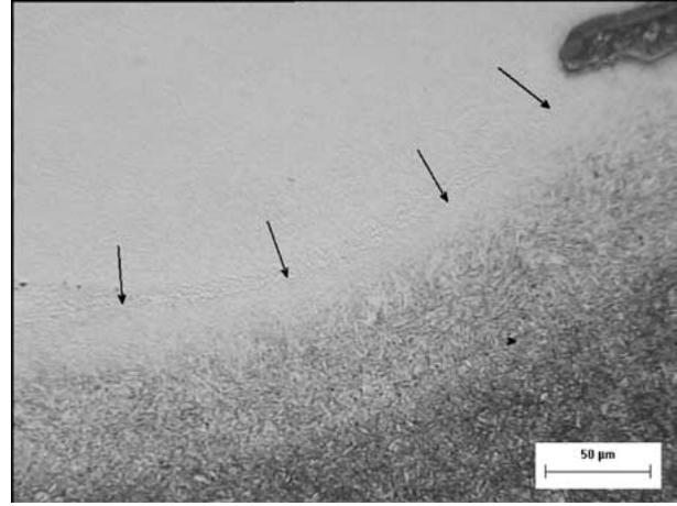
Figure 6 Microstructure of single-pass laser weld HAZ of the 1.2343 steel grade. Arrows indicate the fusion line location.
