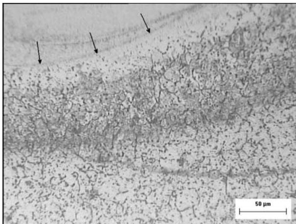
Figure 5 Microstructure of single-pass laser weld HAZ of the 1.2083 steel grade. Arrows indicate the fusion line location.
