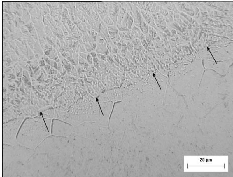
Figure 7 Microstructure of the 1.2343 steel GTAW fusion line region. Arrows indicate the fusion line location.
